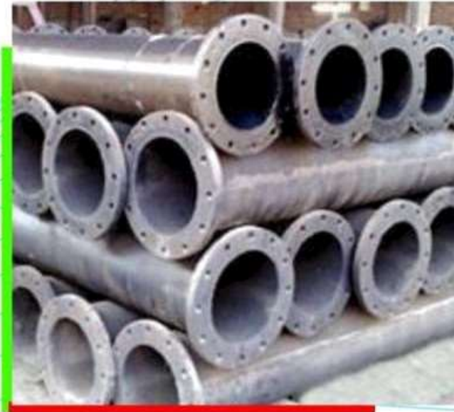
CI pipes- cast iron pipes
